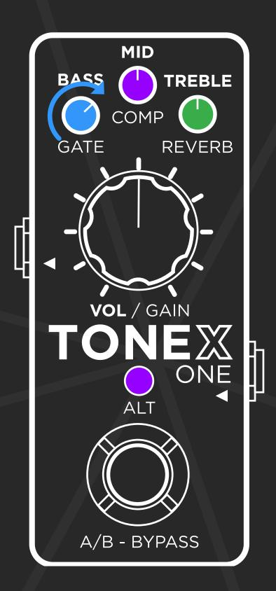
To change the preset loaded in the selected slot, turn the corresponding micro knob. The micro knob will change color according to the selected preset.
